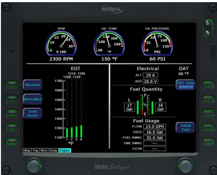
FlightMax Entegra's EMax Total Engine Management™ system provides a graphical fuel totalizer, a lean assist mode, and a percent power display, which take the guess work out of fuel and power management. EMax monitors fuel flow and displays nautical miles per gallon, fuel remaining, fuel to waypoint, and fuel to destination. Temperatures, pressures, RPM, fuel flow, OAT, and electrical bus voltages are also monitored and displayed. EMax provides the most intuitive engine performance monitoring and analysis capability available for G.A.
